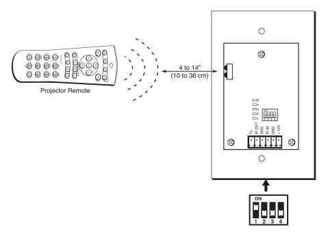
Aiming a projector remote control at the MLC IR learning LEDs
